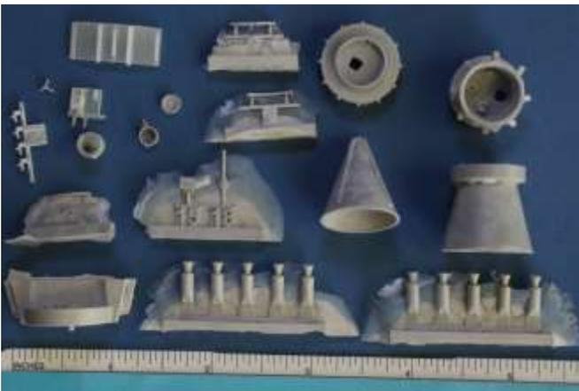
*Here are the rest of the resin parts, including the main Pioneer IV body pieces. The circled piece isn't actually a part: it's the ID tag for the tiny 3D printed tripod piece to its left.*
