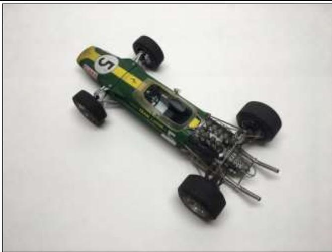
*The 49 was the first F1 car to use the Cosworth DFV 3.0L V8 engine - a design that was used until 1984. It is perhaps the most legendary and successful engine in racing history. The car used the engine as a fully stressed member of the chassis, with the suspension components bolting onto the gearbox. F1 cars use this design philosophy today.*
